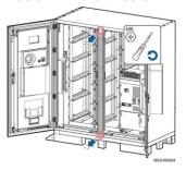
Step 10: Install the air channel plates.
