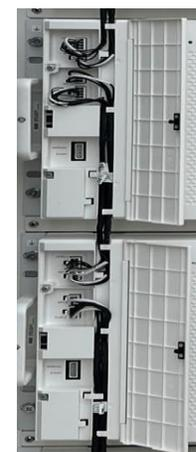
Connecting COM port cables to battery packs
