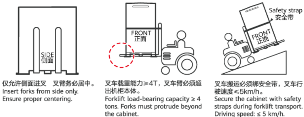
Figure 3-1 Loading and unloading requirements
