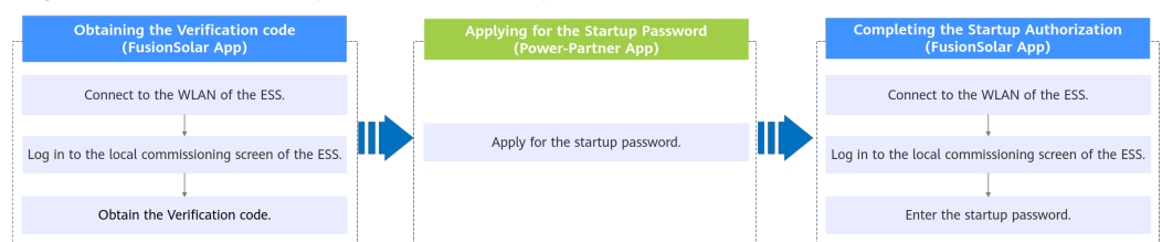
Figure 9-2 ESS startup authorization procedure
